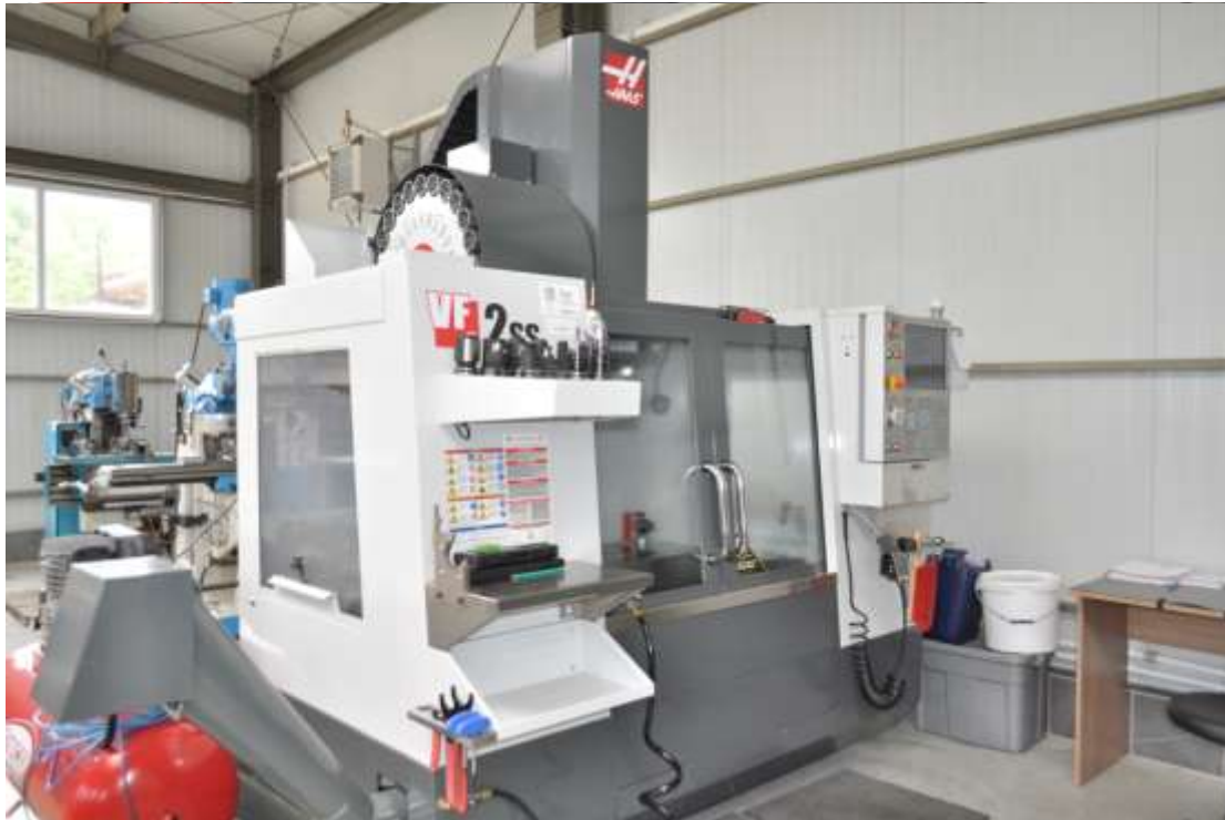
HASS – 4 Axes CNC MILL – super speed 12000 rpm
